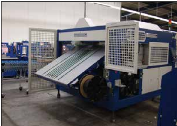
Tilt-up exit table provides excellent working access to sealing head for cleaning and servicing.
