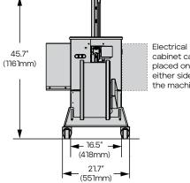
cabinet can be placed on either side of the machine
