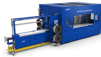
MAX-Q main chassis with a TS-6 Strapper pulled out on transfer cart.
