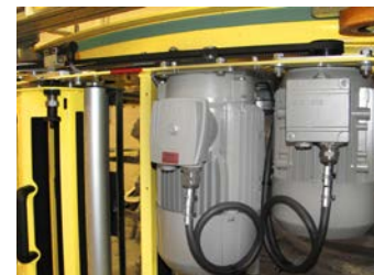
EPS: Electronic Pre-Stretch System
