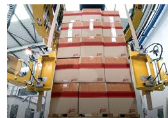
ACBA: Automatic Corner Board Application
