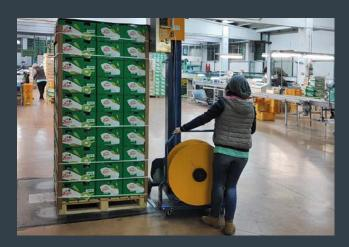
Anyone can strap pallets with the same tension at all strapping heights with this machine.
